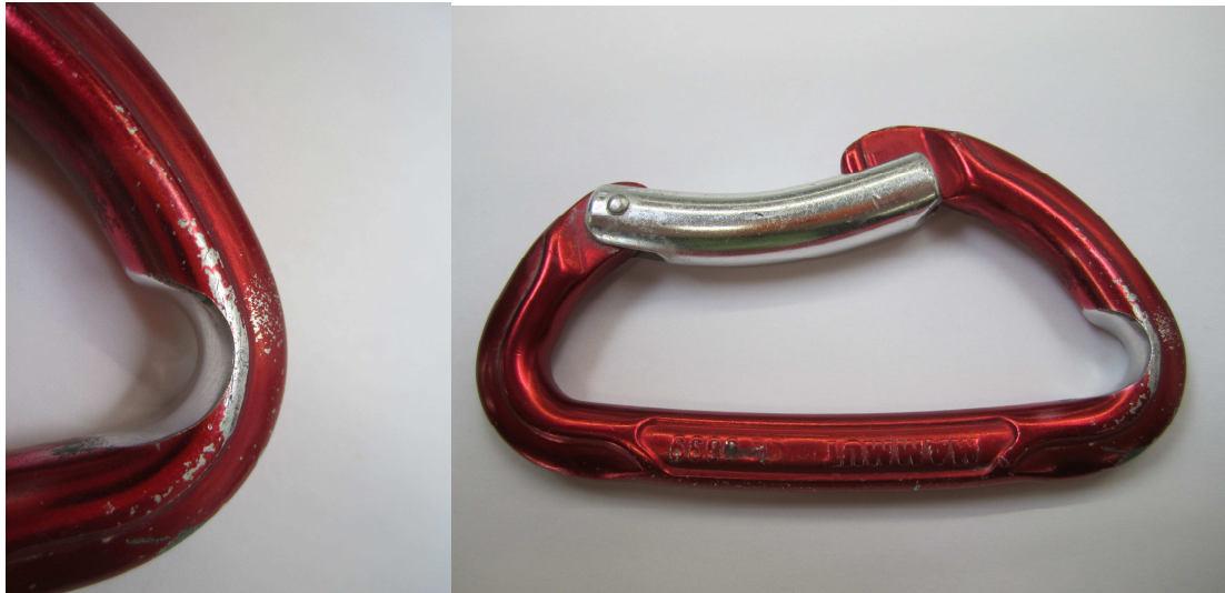
Figure 1: carabiner with sharp edges created through friction from climbing ropes.
